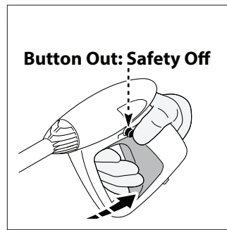
6. Push on the right side of the spray gun to unlock trigger.
