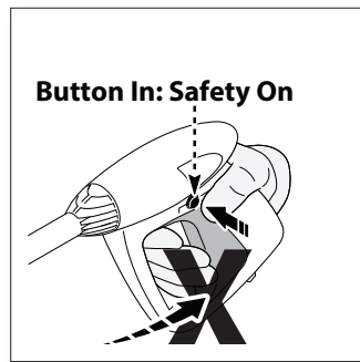
5. Push on left side of spray gun to lock trigger. Always make sure that spray gun is locked when not in use.
